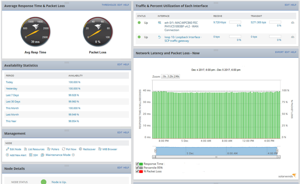
Bandwidth & Network Latency Monitoring Example
